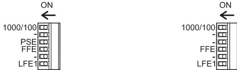
DIP Switches on RLMCSFP24DC, RLMCSFP48DC, and RLMCSFPPOEHO Models
