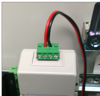
Green Terminal Connector attached to Power Injector
