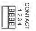
The four CONTACT switches on the front of the unit set the operating mode of the CONTACT OUT terminal pair.
