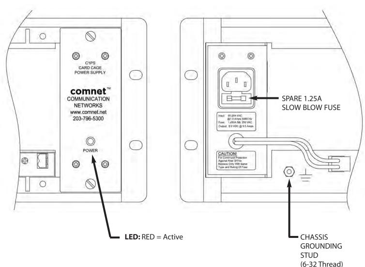
\* The **C1PS** is intended to be installed in the Comnet **C1 Card Cage** only. Any other applications **are not** supported.
