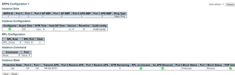
Figure 12 - ERPS 1 (Switch 1) Configuration
