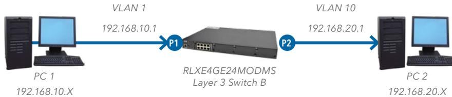
Two PCs in different subnets, use static route function for routing between the two subnets.
