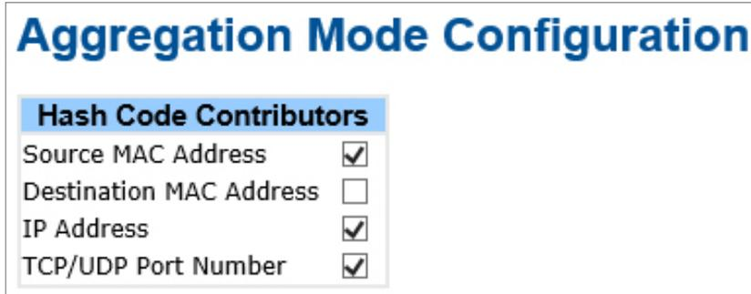
This page is used to configure the Aggregation hash mode and the aggregation group.
