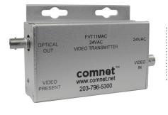
The ComNet™ FVT11MAC video mini-transmitter supports transmission of a fixed video signal using AM modulation on one multimode fiber optic cable. The FVT11MAC video transmitter is compatible with the FVR11M, FVR10M, FVR21, and FVR22 receivers. Plug-and-play design ensures ease of installation requiring no electrical or optical adjustments.
